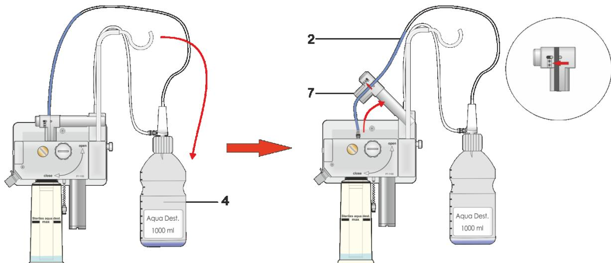
Fig. 120: Turning the water bottle and removing the connection piece
