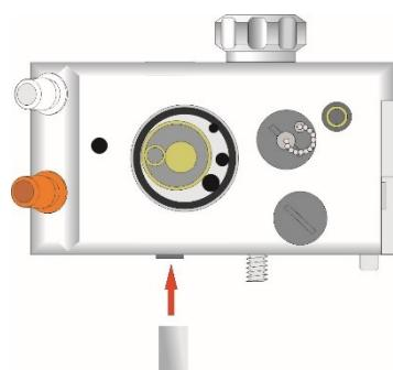
Fig. 167: Attaching the proportional valve's piston
