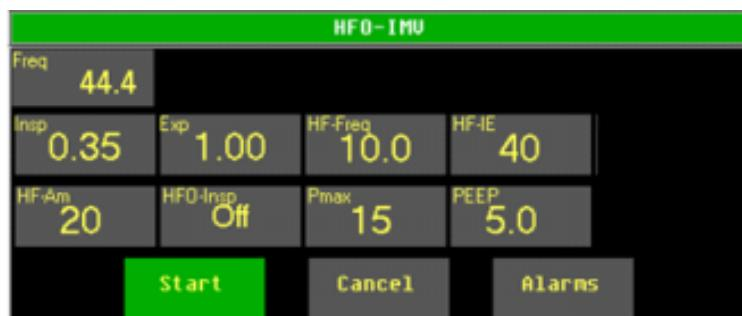
Fig. 87: Parameter settings for HFO with IMV
