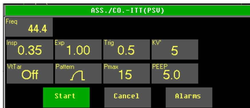
Fig. 85: Parameter settings for Ass./Co. with ITT (PSV)
