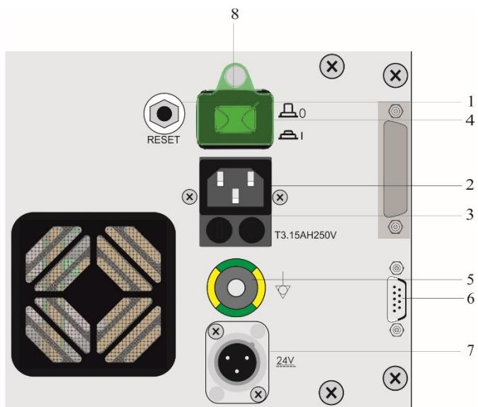
Fig. 28: Power supply module (art. no. 10386120 and art. no. 103861080)
