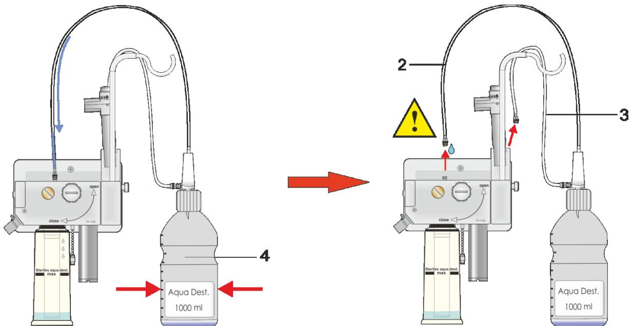
Fig. 121: Back siphoning the residual water and removing the connection piece
