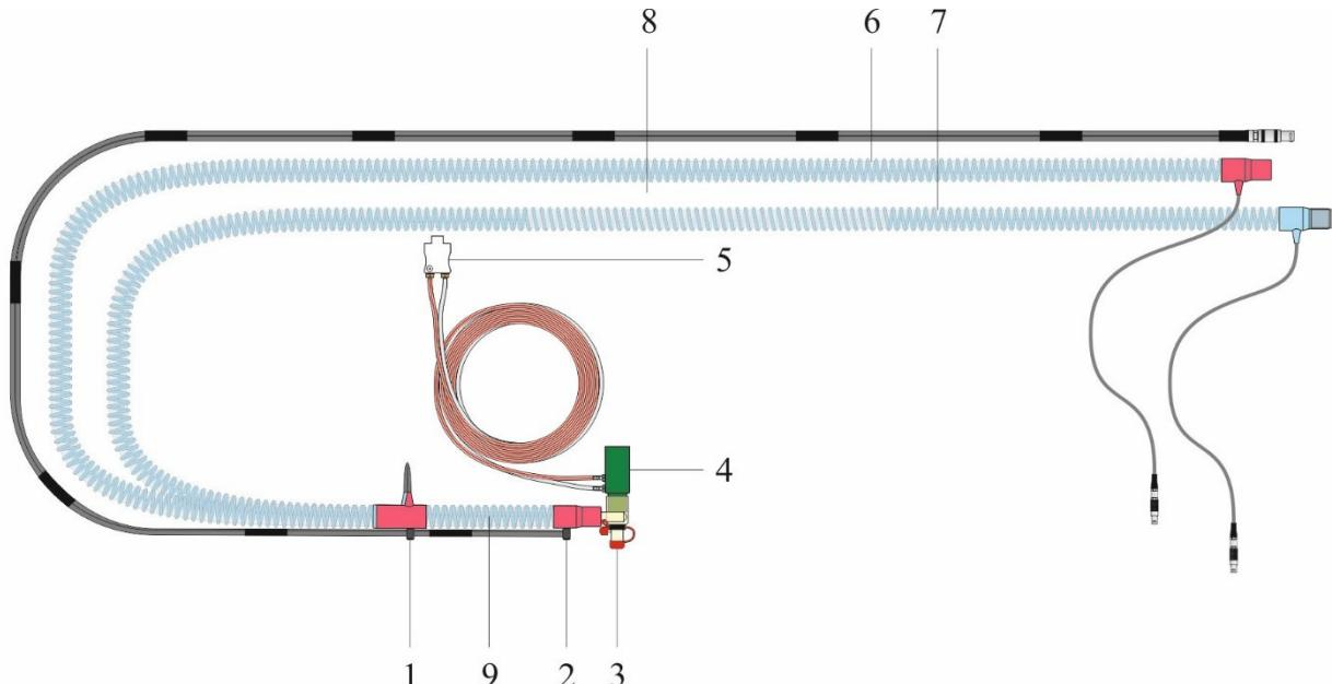
Fig. 22: Tube system for warming beds (art. no. 100761550)
