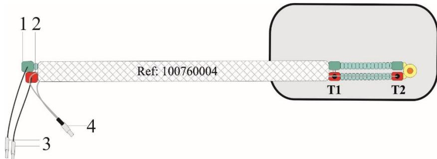
Fig. 145: Using the tube warmer 100760004
