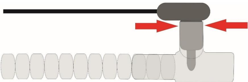
Fig. 107: Inserting the temperature sensor into the adapter
