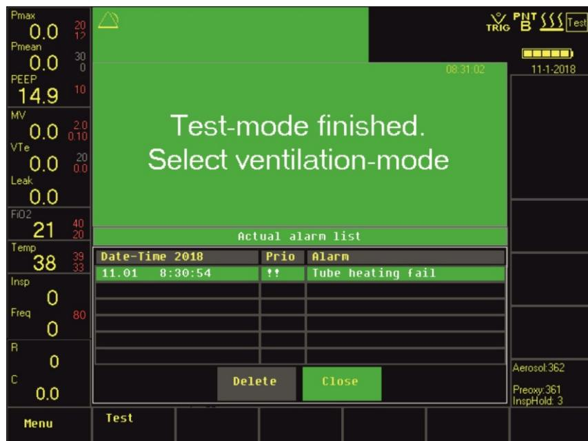
Fig. 73: Test-mode finished, alarms sounded are automatically displayed
