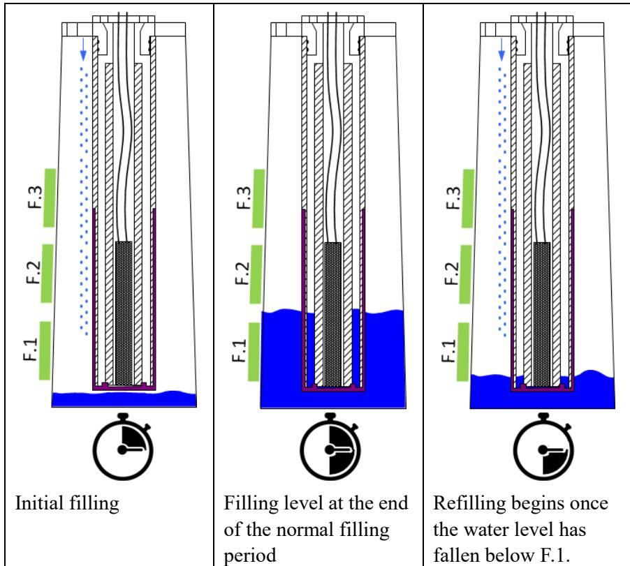
Fig. 147: Automatic refilling with the refill system
