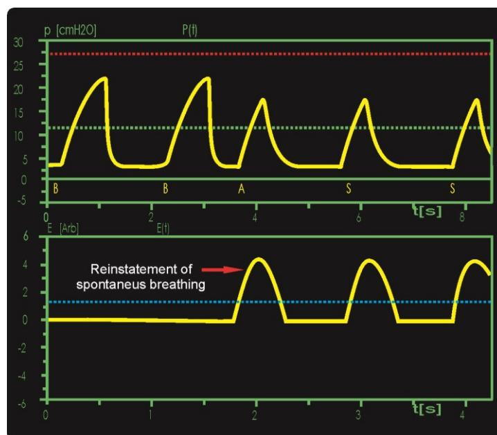
Fig. 137: SNIPPV standard backup mode
