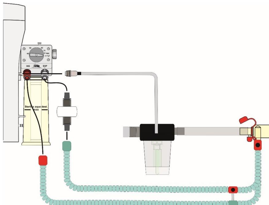
Fig. 112: Installing the pneumatic medication nebulizer
