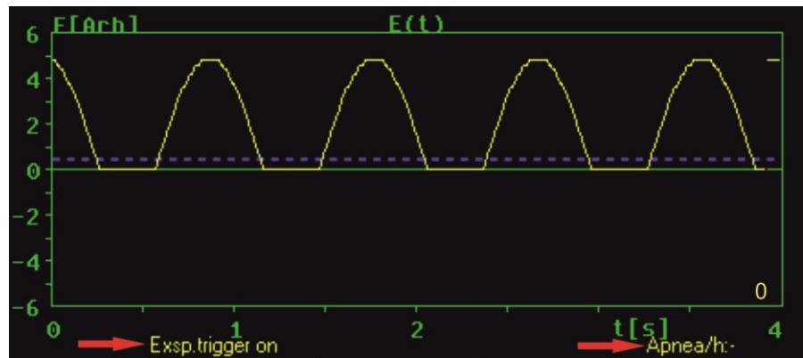
Fig. 17: External expiratory trigger status and apnea counter
