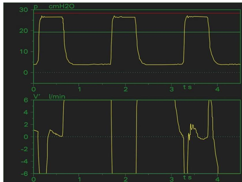
Fig. 150: Humidity in the pneumotachograph
