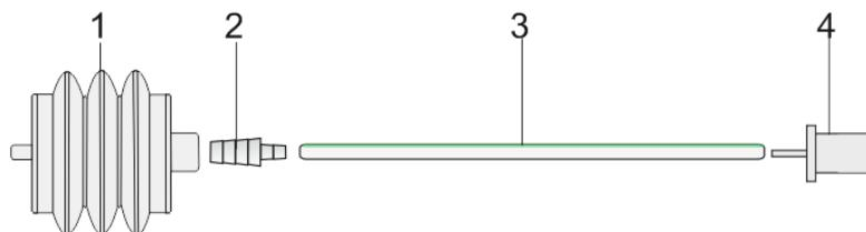
Fig. 165: Test lung with tube adapter
