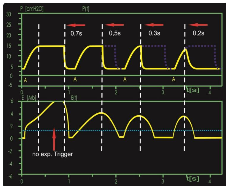
Fig. 135: Expiratory trigger during SNIPPV
