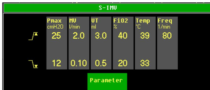
Fig. 64: Setting alarm limits
