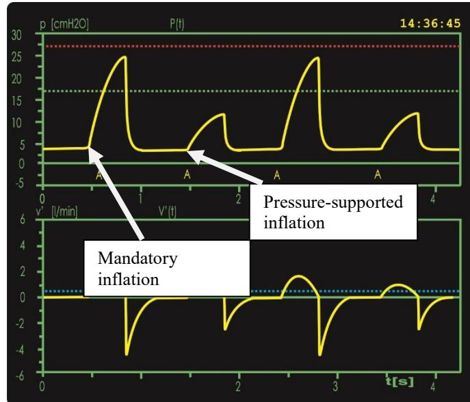
Fig. 125: SIMV with ITT and pressure support
