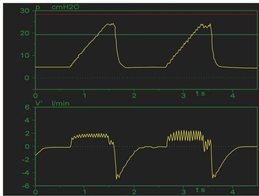
Fig. 149: Oscillating ventilation curves – patient valve
