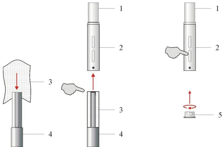
Fig. 100: Inserting the humidifier fleece
