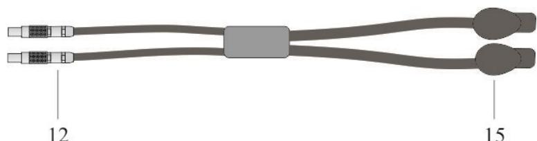
Fig. 156: Connection cable P3/P7 for disposable patient tube system
