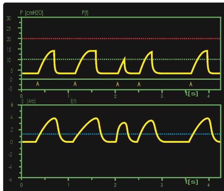
Fig. 134: Pressure support during SNIPPV
