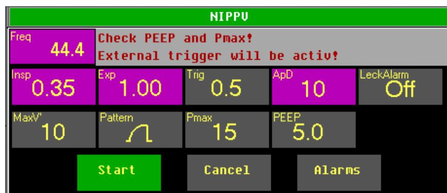
Fig. 94: Parameter settings for NIPPV (with frequency-controlled backup ventilation)
