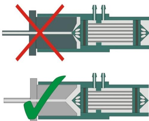
Fig. 108: Tube adapter
