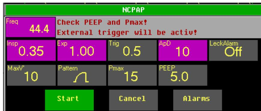
Fig. 91: Parameter settings for NCPAP (with frequency-controlled backup ventilation)
