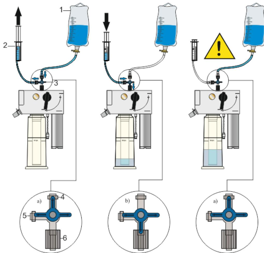
Fig. 101: Filling the humidifier bottle
