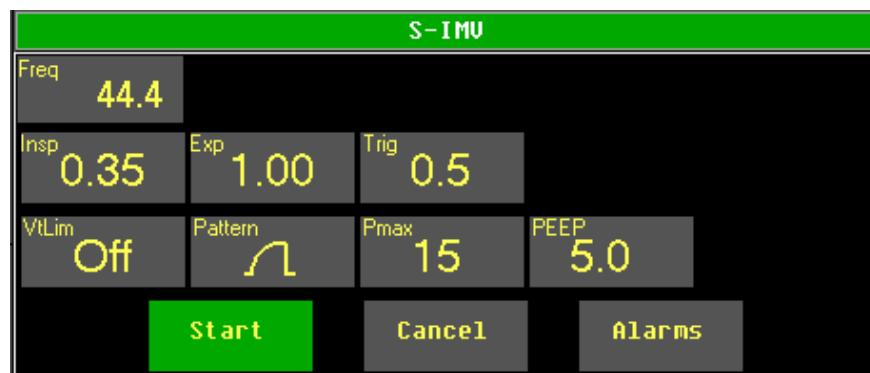
Fig. 62: Starting ventilation
