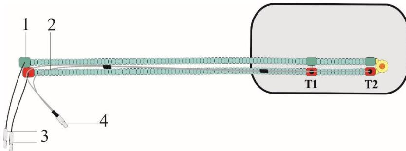
Fig. 105: Sensor position with tube system for warming bed
