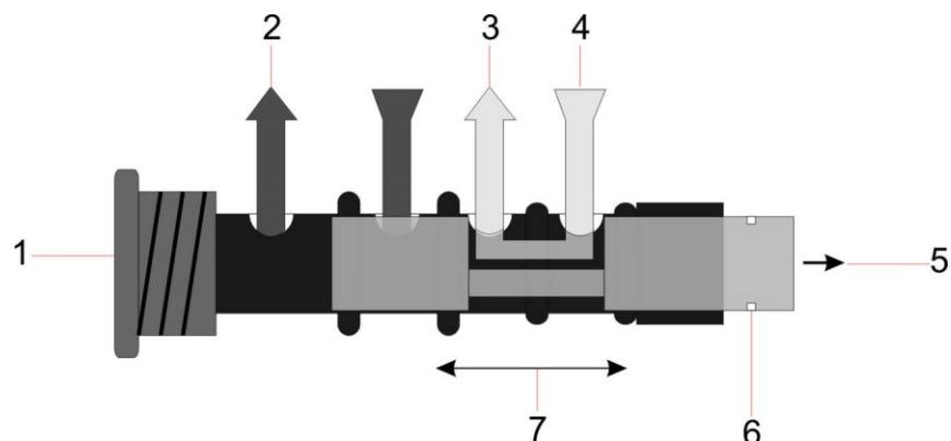
Fig. 146: Patient valve P7, valve piston in the inspiration position
