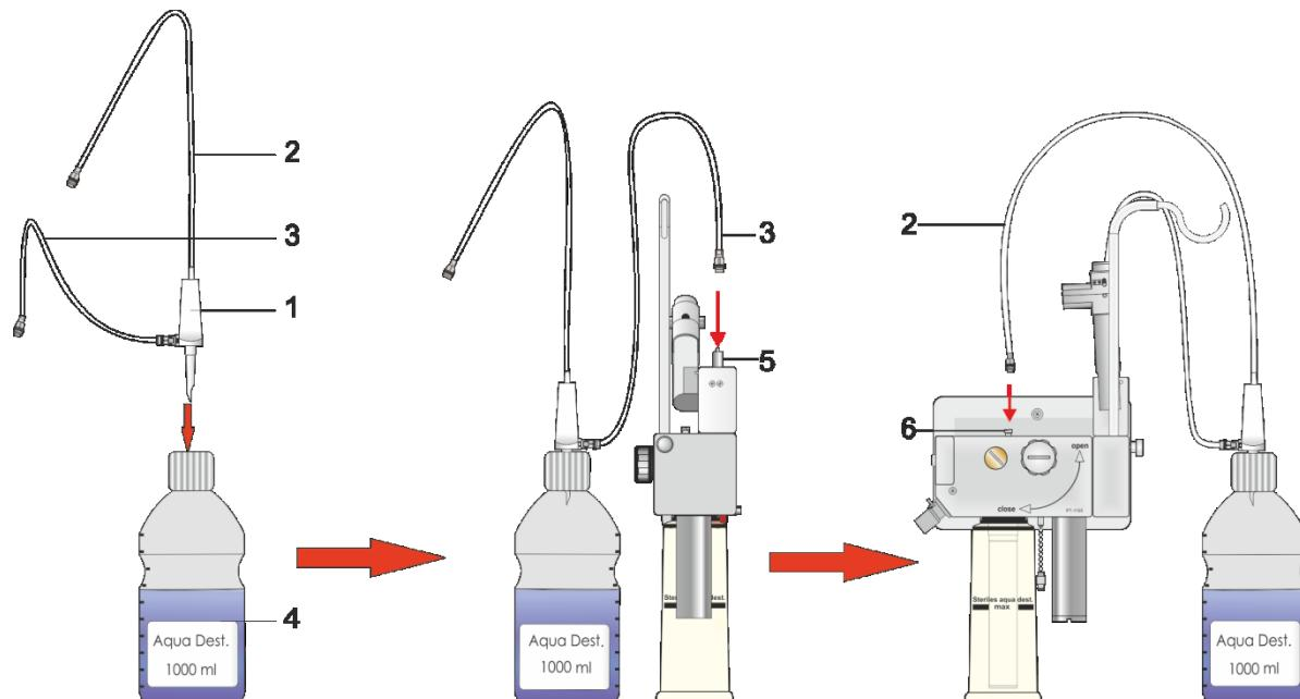
Fig. 102: Installing the water bottle and connection piece
