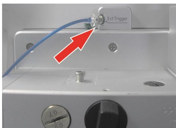
Fig. 113: Connection of the external respiration sensor
