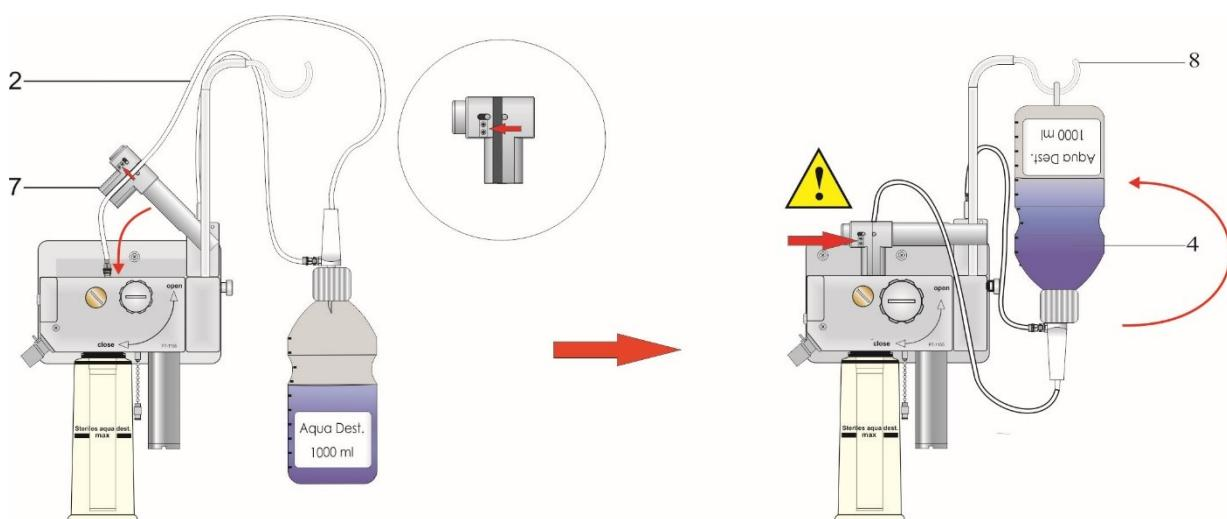
Fig. 103: Inserting the connection piece in the pinch valve
