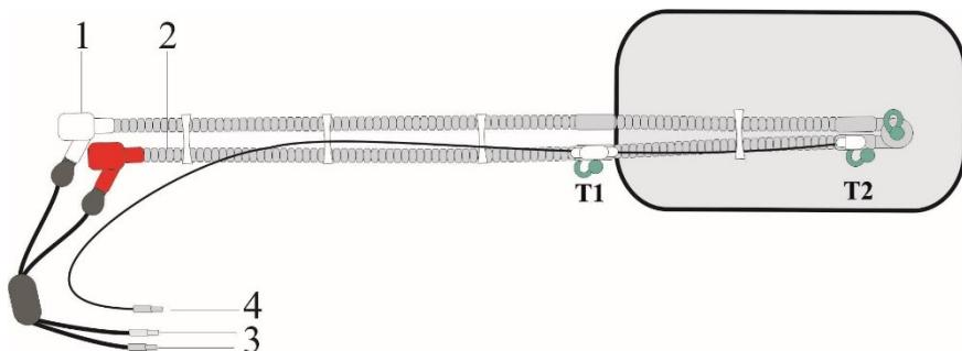
Fig. 106: Sensor position with disposable patient tube system
