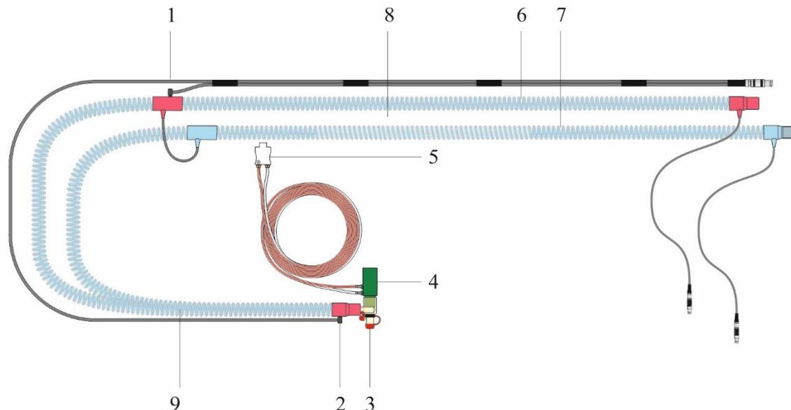
Fig. 21: Tube system for incubators (art. no. 100761500)
