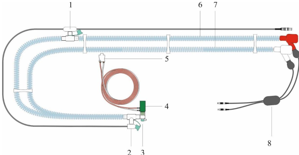
Fig. 23: Disposable tube system P3/P7 (art. no. 100761300)
