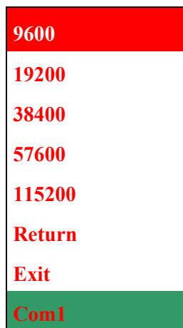
Fig. 55: Selecting the transmission speed
