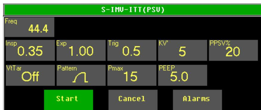
Fig. 81: Parameter settings for S-IMV-ITT (PSV)
