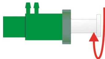
Fig. 163: Inserting the assembly tool and rotating slightly
