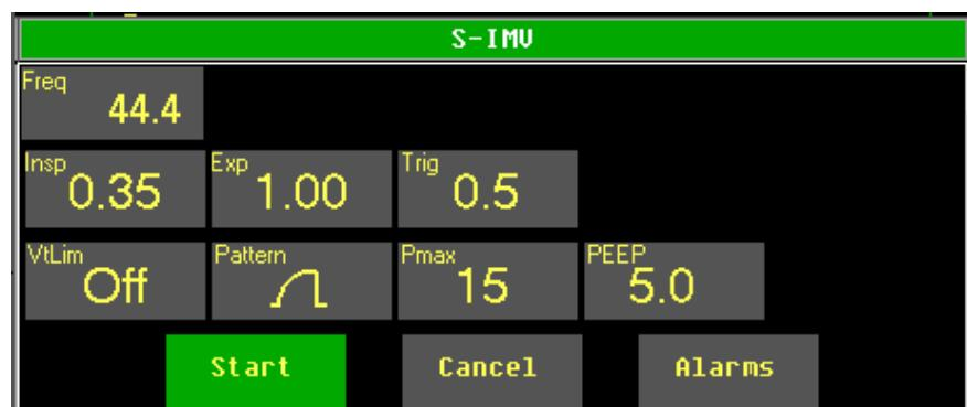
Fig. 79: Parameter settings for S-IMV
