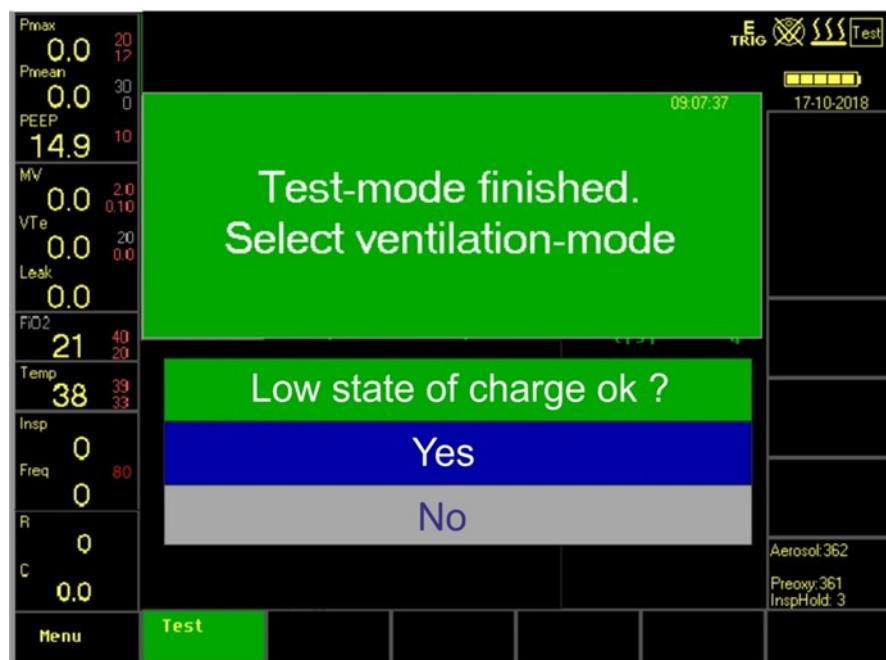
Fig. 117: Operation with low battery charge level
