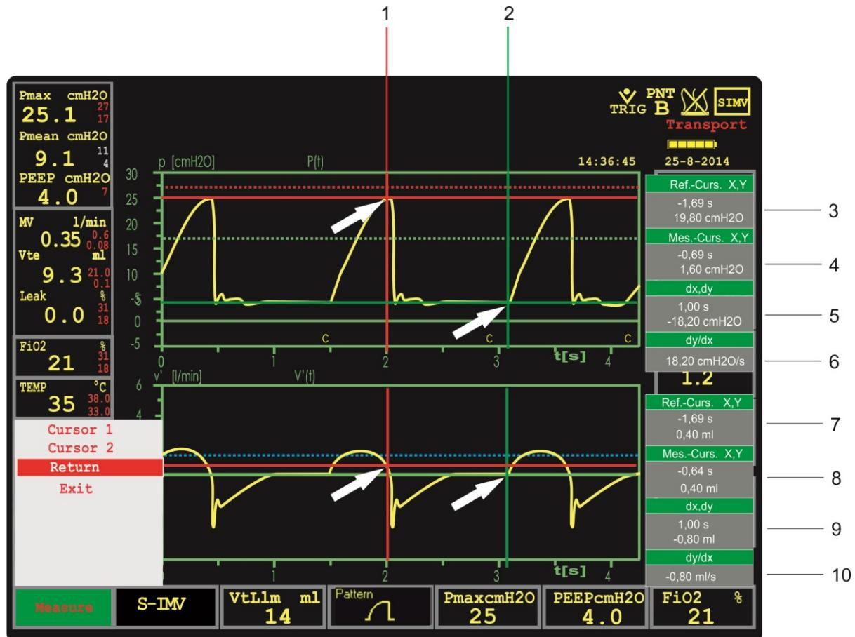
Fig. 44: Measure menu (arrows show the measured points)
