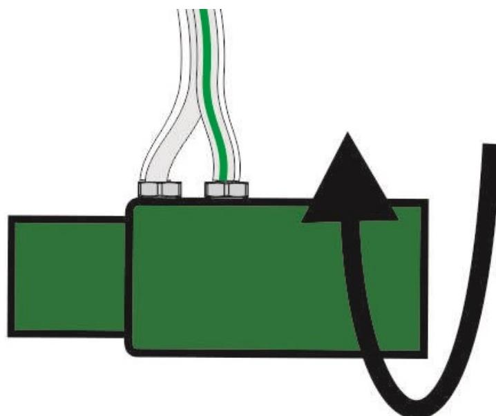
Fig. 152: Turning the measuring tube connectors upward
