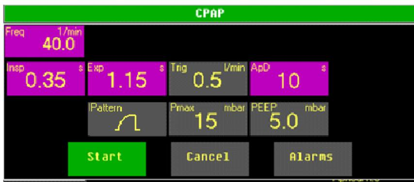
If the ventilation mode is changed to CPAP, the ventilation pattern »SINUS« is preset automatically, but only used for the special function »Insp. Hold« and for optional backup ventilation. The pattern can still be modified if needed.
