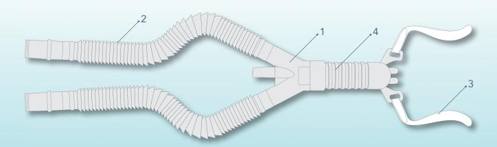
Firstly, the y-shaped applicator (1) is connected to the decoupling tubes (2). After this the two fixing straps (3) are fastened to the prong (4).
